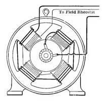
FIG. 57. Diagram of compound field excitation as used in most d. c. generators and in some d. c. motors.
